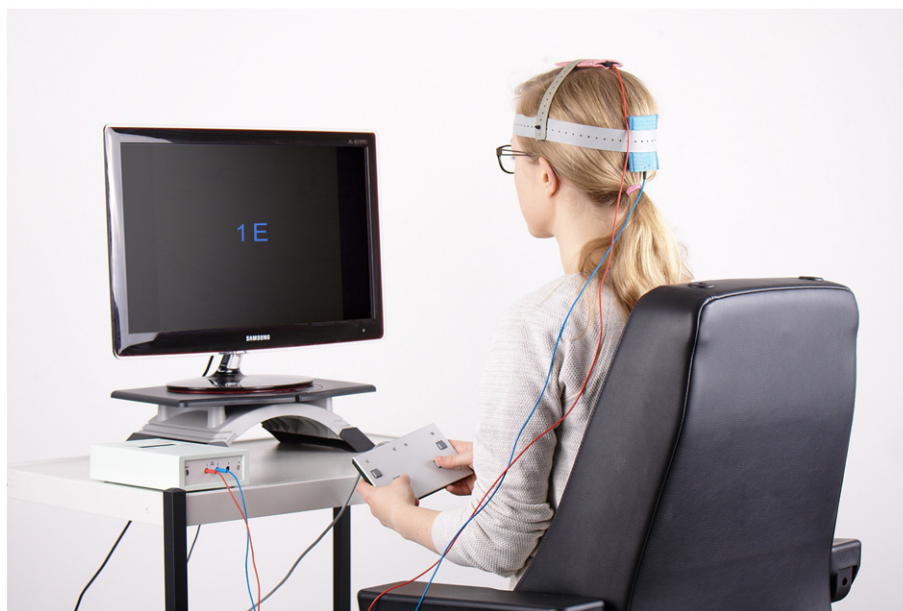
Fig. 5. Transcranial electric stimulation (TES). TES delivers an electric current directly to the human scalp, some of which passes through the skull and interacts with neural activity. At least two electrodes are used that received their names from tDCS: an anode (red electrode at top of head) and a cathode (blue electrode over back of head). For tACS, this terminology is misleading and recent paradigms employ multiple smaller electrodes for increased spatial resolution.
