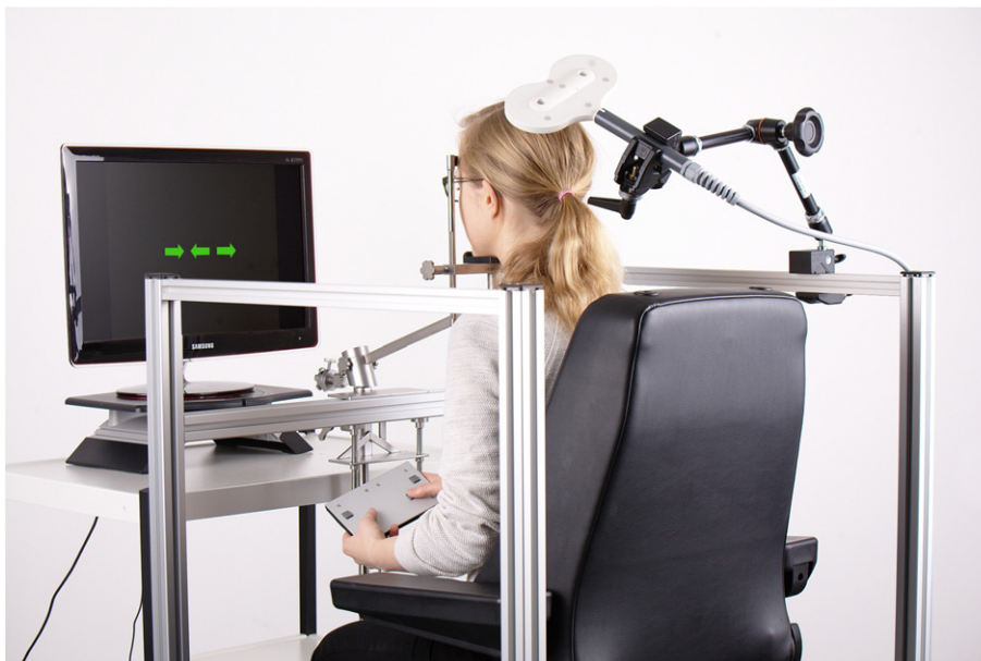
Fig. 4. Transcranial magnetic stimulation (TMS). TMS delivers one or multiple magnetic impulses to the human head via a coil that often has a figure-eight shape. The magnetic field passes the skull and induces an electric current that interacts with neural activity. Here, the subject is performing a task on the screen while being stimulated.
