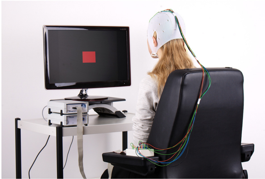
Fig. 3. EEG-neurofeedback. In order to have subjects learn how to control a parameter of their EEG, this parameter has to be visualized and fed back to the subject. Usually, only a subset of the 32 or 64 electrodes is used for this purpose. Here, the amplitude of the frontal midline theta from a few frontal midline electrodes is fed back via a computer screen. Red or blue squares indicate an increase or decrease of theta amplitude as compared to a baseline, respectively.
